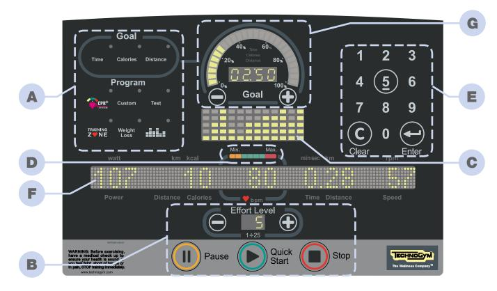
A <u>Function keys</u> for workout or test selection. If the corresponding LED lights up, this key is active or the corresponding exercise is in progress.
