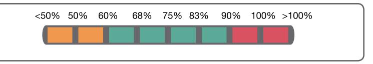
The first two LEDs, coloured orange, signal a heart rate less than 60% of the theoretical maximum heart rate; the four central LEDs, coloured green, signal values between 60% and 90%; the two red LEDs signal a heart rate greater than 90%.
